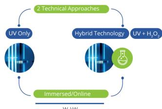
There are different possible disinfection methods: submerged (in the basin or tank) or in-line (outside of the your installations, etc.
